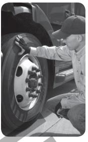
inflation increases the rolling resistance of radial tires, which means higher fuel costs and less tread life. Tread separation, bruises, breaks, and blowouts can result.
