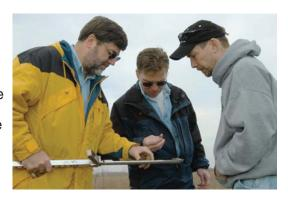
soil types at an excavation site. Soil classification is used to determine the need for a protective system.
