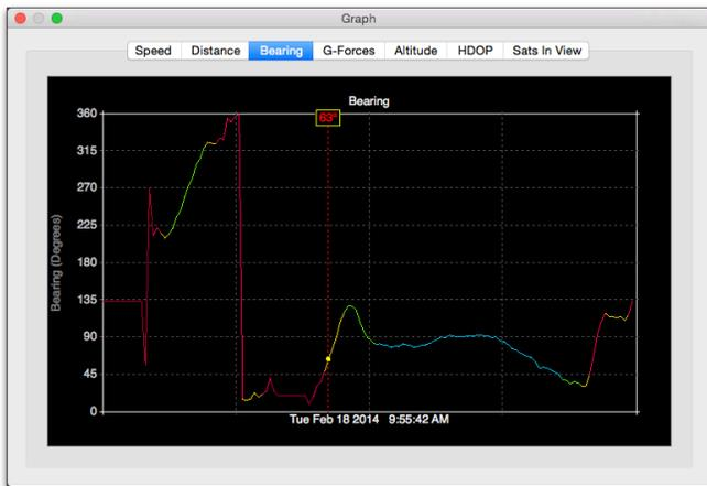
The **Bearing** graph shows the history of direction for the vehicle. North is 0 or 360-deg, East is 90-deg, South is 180-deg, and West is 270-deg.
