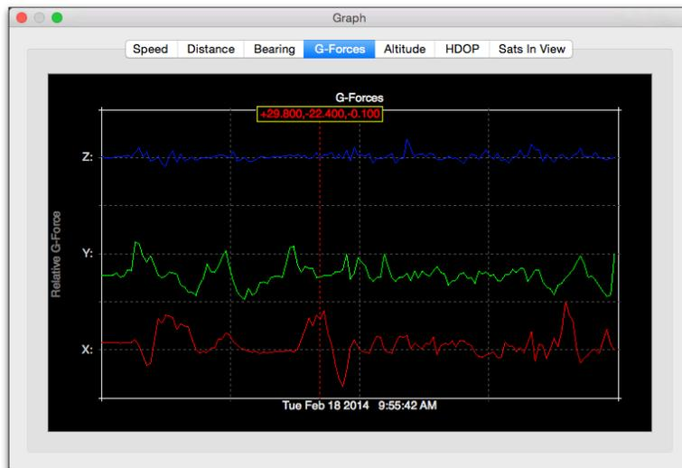
The **G-Forces** graph displays the X, Y, and Z components of acceleration from the dashcam's shock sensor. The G units vary from manufacturer to manufacturer so the plots should be considered relative G-force. The X and Y components are horizontal force and the Z component is vertical. The 1-g effect of gravity is subtracted from the Z component in the graph
